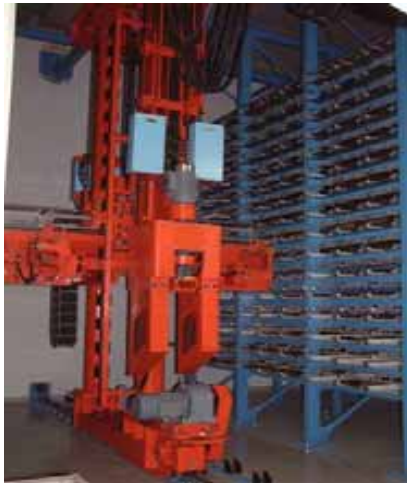
Stacker crane type automated intermediate pin storage
