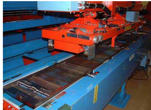
Each fabrication station is connected by fully automated fuel pins transferring conveyer system
