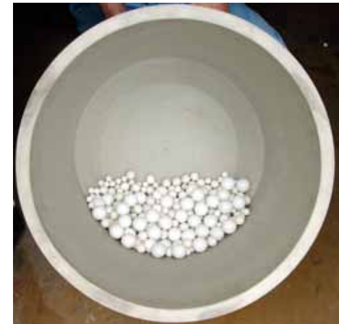
\text{Al}_2\text{O}_3 balls & Si rubber lining
